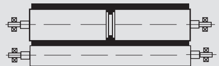
4. Belt with internal tracking guide supported by a cylindrical roller and driven by a grooved driving pulley.
