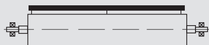
1. Belt with cleats (flights) in "V", section supported on a cylindrical roller.
