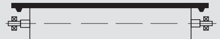
5. Belt with sidewalls supported by a cylindrical roller which is narrower than the belt.
